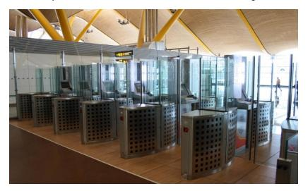
this setup travelers access the lock gate through the first door, proceed with the identification inside and access the airport terminal through the second door that opens automatically after positive verification of the citizen's identity. The VeriLook facial recognition engine is used for face matching, as all passports include an individual's facial image. VeriFinger is used for fingerprint matching with all 2<sup>nd</sup> generation European
