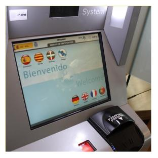
system performs a more secure dual-biometric test using facial and fingerprint recognition. It is for this multi-biometric verification that Indra has chosen the Neurotechnology product line.
